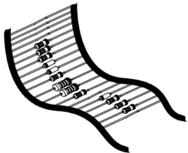
**AXIAL COMPONENTS ARE TAPED IN THE CORRECT MOUNTING SEQUENCE !**
