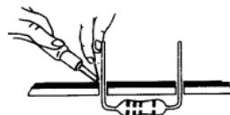
2- Make sure the solder joints are cone-shaped and shiny
