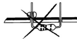
3- Trim excess leads as close as possible to the solder joint
